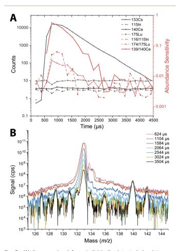
Fig. 3 (A) Average signal from individually detected droplets containing 5 μg mL<sup>-1</sup> Cs and a nebulized solution containing 1 ng mL<sup>-1</sup> In, Ce, and Lu (black). Average abundance sensitivity of In, Ce, and Lu across the Cs droplet profile (red). Data was recorded with a 48 µs time resolution. (B) Mass spectrum at different time intervals across the droplet profile. This demonstrates the transient long range baseline elevation from an intense particle signal.
