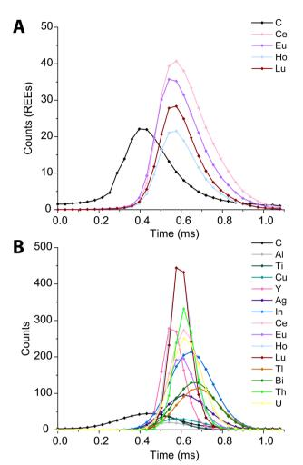
Fig. 6 Average time trace profiles for 1200 REE-doped polystyrene beads (A) and 2000 microdroplets containing 100 ng mL $^{-1}$  metals and 100  $\mu$ g mL $^{-1}$  carbon (B) acquired with a time resolution of 36  $\mu$ s.
