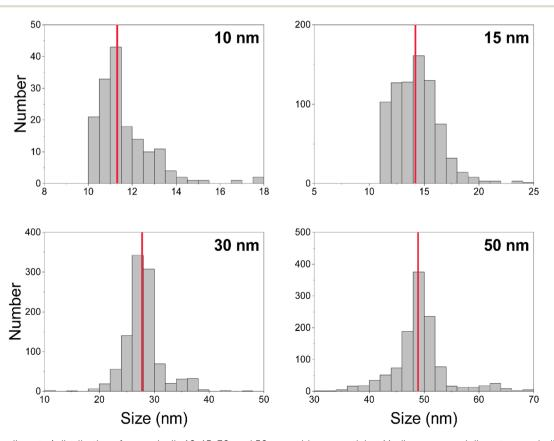
Fig. 4 Size (i.e. diameter) distributions for nominally 10, 15, 30, and 50 nm gold nanoparticles. Median measured diameters are indicated by the red lines and are as follows (left to right, top to bottom): 11.8 nm, 14.2 nm, 27.8 nm, 48.9 nm.
