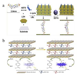
Fig. 3 (a) Schematic of fluorimetric Cd2+ detection using an ultrathin film from ZnAl-LDH nanosheets and ABTS. Reprinted with permission from ref. 54. Copyright 2011, American Chemical Society. (b) Schematic illustration of fluorescence turn-on Cr(vi) based on Fe(CN)<sub>6</sub><sup>4-</sup>-intercalated NiAl-LDHs and TA. Reprinted with permission from ref. 58. Copyright 2020, Elsevier.
