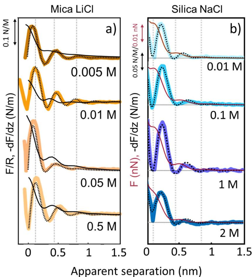
Fig. 3 Averaged ( $n = 80$ ) force gradient ( $-dF/dz$ ; thick lines) and force ( $F$  thin dark red lines on silica and  $F/R$  thin black lines on mica) versus apparent tip–sample separation of various concentrations of  $\text{LiCl}$  on mica (a) and of  $\text{NaCl}$  on silica (b). Each salt was measured with a separate AFM tip at pH 6. Dashed lines: empirical fits to eqn (1).
