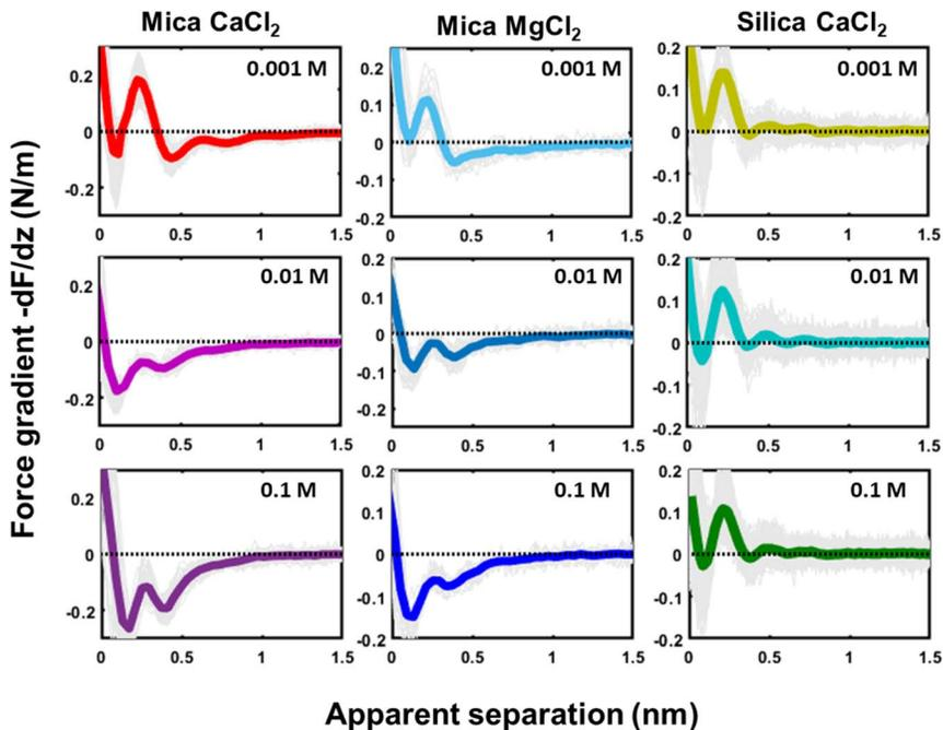
Fig. 4 Force gradient ( $-dF/dz$  ( $\text{N m}^{-1}$ ) versus apparent separation (nm) measured in 1, 10 and 100 mM of  $\text{CaCl}_2$  and  $\text{MgCl}_2$  on a mica substrate and of  $\text{CaCl}_2$  on a silica substrate. The thin gray lines are individual measured curves, the thick line is the average of these lines. The measurements at the mica and silica substrate are obtained with different tips at pH 6.
