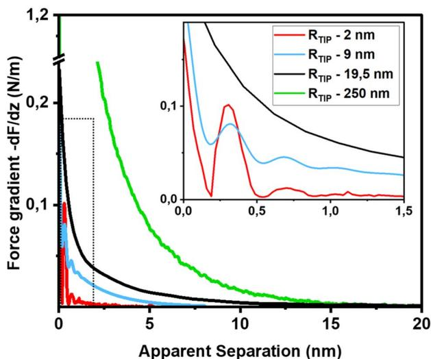
Fig. 5 Force gradient vs. separation curves on smooth silica surfaces recorded with AFM tips of different size (10 mM NaCl solution; pH 6). Solid red line: same data as in Fig. 3b (tip radius ( $R_{\text{TIP}}$ )  $\approx 2$  nm); blue line: from ref. 36 (tip radius: 9 nm); black line (tip radius: 19.5 nm); green line from ref. 56 (tip radius: 250 nm). The SEM and HR-TEM images of the AFM tips are shown in ESI Fig. S16.†
