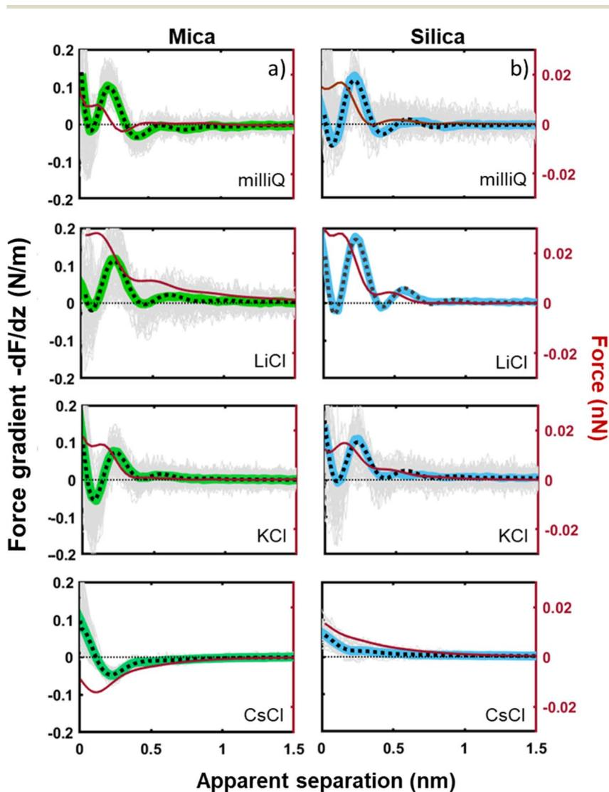
Fig. 2 Averaged force gradient ( $-dF/dz$ ; thick green lines for mica and thick blue lines for silica) and force ( $F$  thin dark red lines) versus apparent tip–sample separation measured in pure water (top panel; light grey: 180 individual force curves) and for various salt solutions at a fixed concentration of 50 mM. All the data were recorded with the same AFM tip at pH 6. Dotted lines: empirical fits to eqn (1).
