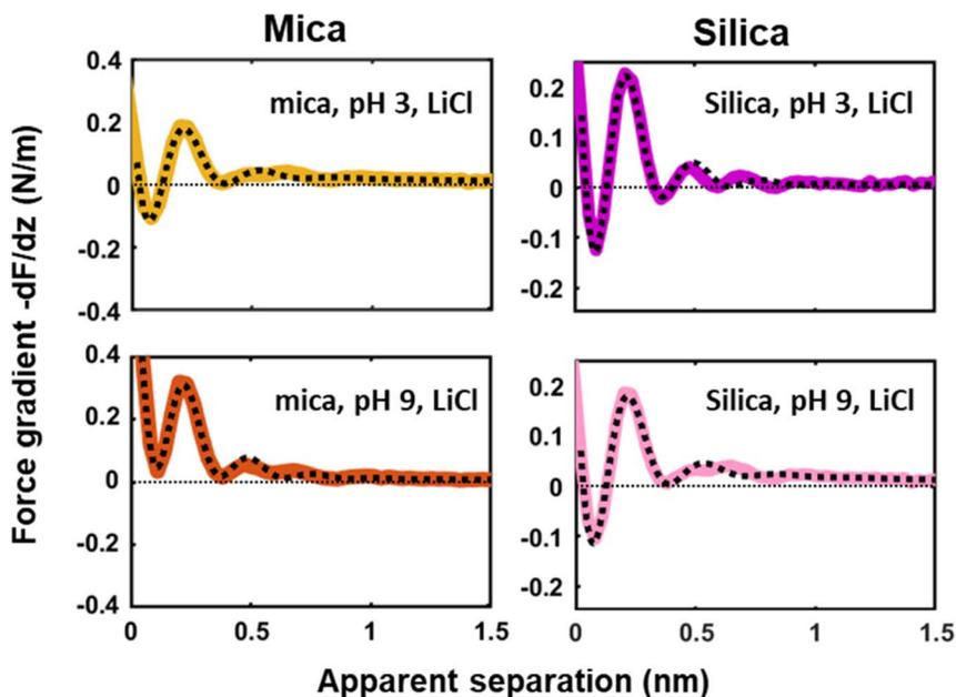
Fig. 6 Averaged ( $n = 100$ ) force gradient ( $-dF/dz$ ; colored thick lines) versus apparent tip-sample separation measured in 50 mM LiCl solutions, with bulk pH values of pH 3 and 9, on a silica and mica substrate. The pH was adjusted by adding either HCl or NaOH. The data shown here were collected using the same AFM probe. The dotted lines represent the fit using eqn (1).
