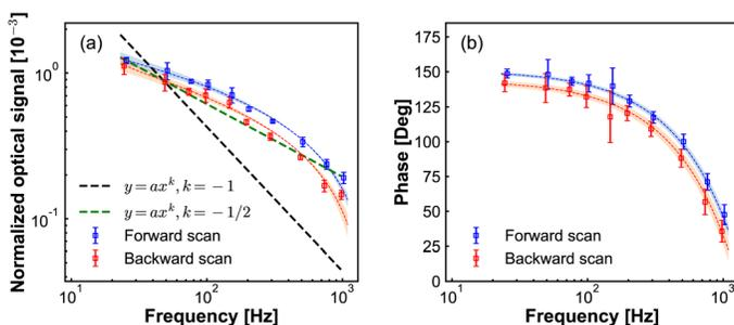
Fig. 5 Normalized optical amplitude (a) and phase (b) signals from lock-in amplifier with different frequency of potential modulation. DC potential scan from  $-200$  mV to  $300$  mV with a scanning rate of  $50$   $\text{mV s}^{-1}$ , the amplitude of potential modulation is  $50$  mV, and the concentration of  $\text{Fe}(\text{MeOH})_2$  is  $15$  mM.
