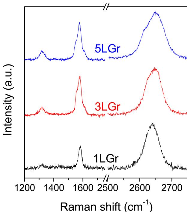
Fig. 1 Raman spectra of the 1-, 3- and 5-layers graphene samples on Si/SiO<sub>2</sub> wafer, denoted 1LGr, 3LGr and 5LGr, respectively.
