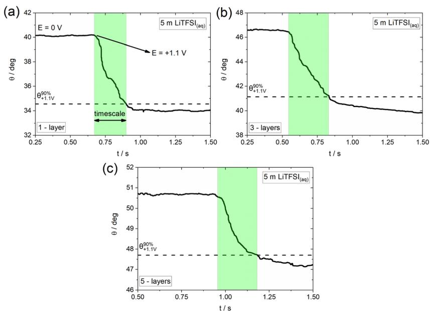
**Fig. 4** Change in apparent contact angle,  $\theta$ , and timescales (highlighted regions) during a wetting cycle in 5 m LiTFSI<sub>(aq)</sub> following the protocol described in the Experimental section for (a) 1-, (b) 3- and (c) 5-layers CVD graphene. The depicted cycle corresponds to a potential pulse from 0 V to +1.1 V vs. pseudo-Pt, *i.e.*, in the potential region where TFSI<sup>-</sup> anion adsorption/intercalation occurs.
