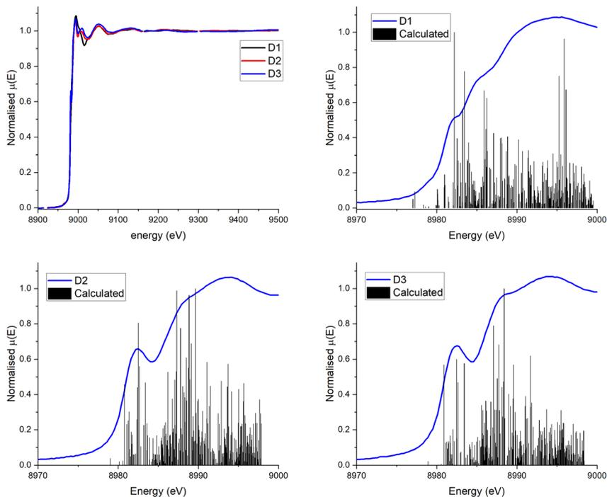
**Fig. 4** (a) Experimental Cu K-edge XANES spectra for **D1** (black), **D2** (red) and **D3** (blue) in MeCN solution at r.t. (b–d) Experimental XANES (blue) and results of preliminary calculations of XANES (black) of complexes **D1–D3**. The energy axis for the calculated spectra has been shifted upwards by 98.25 eV so that the edge corresponds to the edge of the experimental data. Experimental data are average of multiple runs, see Fig. S17† for the data from individual runs.
