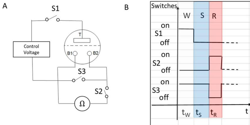
Fig. 2 (A) Memory configuration with a temporary short-cut instead of the bypass used before.<sup>20</sup> (B) Timeline of the writing–storing–reading (W–S–R) protocol.
