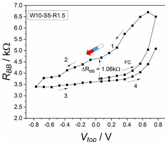
Fig. 3 Writing-voltage dependence of  $R_{BB}$  using the W-S-R protocol. A voltage cycle indicated by the labels FC-1-2-3-4 was measured. We call the data points of the first application of voltage to the cell the formation curve (FC). The colored arrow (white for W, blue for S, and red for R) and the code W10-S5-R1.5 indicate the protocol applied in-between two data points.
