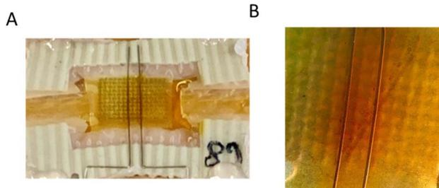
Fig. 7 (A) Coloration difference between the two bottom electrodes after applying  $V_{\text{top}} = -0.87$  V for 1 min. (B) A similar sample under a microscope after applying  $V_{\text{top}} = -0.87$  V for 1 min.
