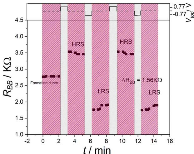
Fig. 5 A switching measurement with the protocol W60–(S20–R1.5)<sub>n</sub>. This means that a voltage is applied on the top electrode for 1 min, then a storing time of 20 s is applied for every reading that is taken.
