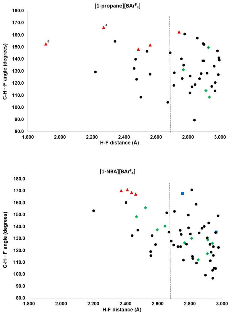
Fig. 4 Scatterplots of H $\cdots$ F distance (Å) vs. C–H $\cdots$ F angle (degrees) for the [1-NBA]<sup>+</sup> and [1-propane]<sup>+</sup> cations within the octahedral arrays of neighbouring [BAR<sup>F</sup><sub>4</sub>]<sup>−</sup> anions. The dashed vertical line indicates the sum of the van der Waals radii for H and F. <sup>a</sup>Data points correspond to two equivalent H $\cdots$ F contacts.
