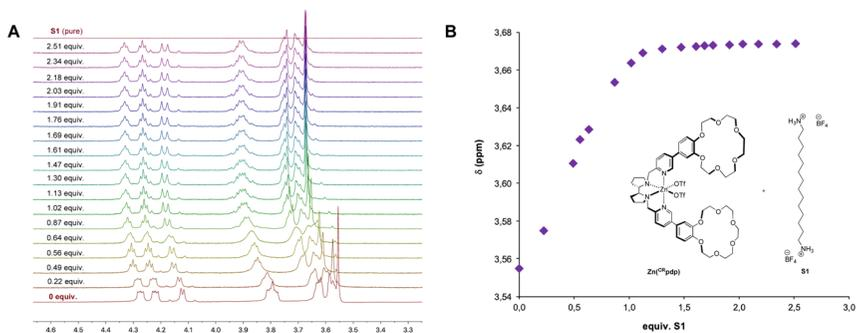
Fig. 2 Binding of **S1** to  $\text{Zn}^{\text{CR}}\text{pdp}$  (1 mM) in  $\text{CD}_3\text{CN}$  at  $25^\circ\text{C}$ . (A) Enlargement of the region between 3.3 and 4.6 ppm, corresponding to the crown ether signals. (B) Titration curve.
