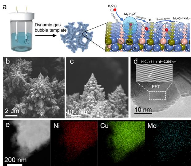
**Fig. 2** Structure characterization of NiCuMo alloy. (a) Schematic of the preparation of the NiCuMo alloy by hydrogen bubble dynamic templated electrodeposition. (b) and (c) The SEM and (d) TEM images of NiCuMo alloy. (e) EDS elemental mapping images.
