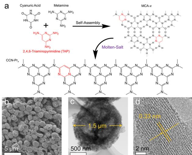
**Fig. 1** (a) The proposed preparation process of CCN-Pr<sub>x</sub>. (b) Scanning electron microscopy (SEM) and (c and d) transmission electron microscopy (TEM) images of CCN-Pr<sub>40</sub>.
