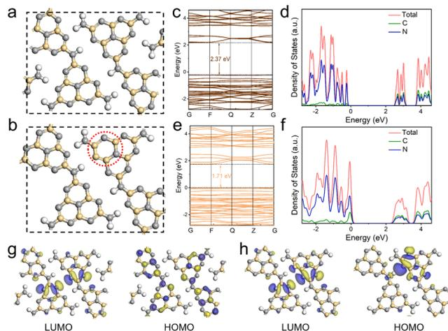
Fig. 4 Structure models of (a) CCN-Pr<sub>0</sub> and (b) CCN-Pr<sub>40</sub>. Calculated band structures and corresponding DOS of (c and d) CCN-Pr<sub>0</sub> and (e and f) CCN-Pr<sub>40</sub>. LUMO and HOMO distributions of (g) CCN-Pr<sub>0</sub> and (h) CCN-Pr<sub>40</sub>. The blue and yellow regions represent the net electron accumulation and depletion, respectively. The gray, yellow, and white spheres represent the N, C, and H atoms, respectively.
