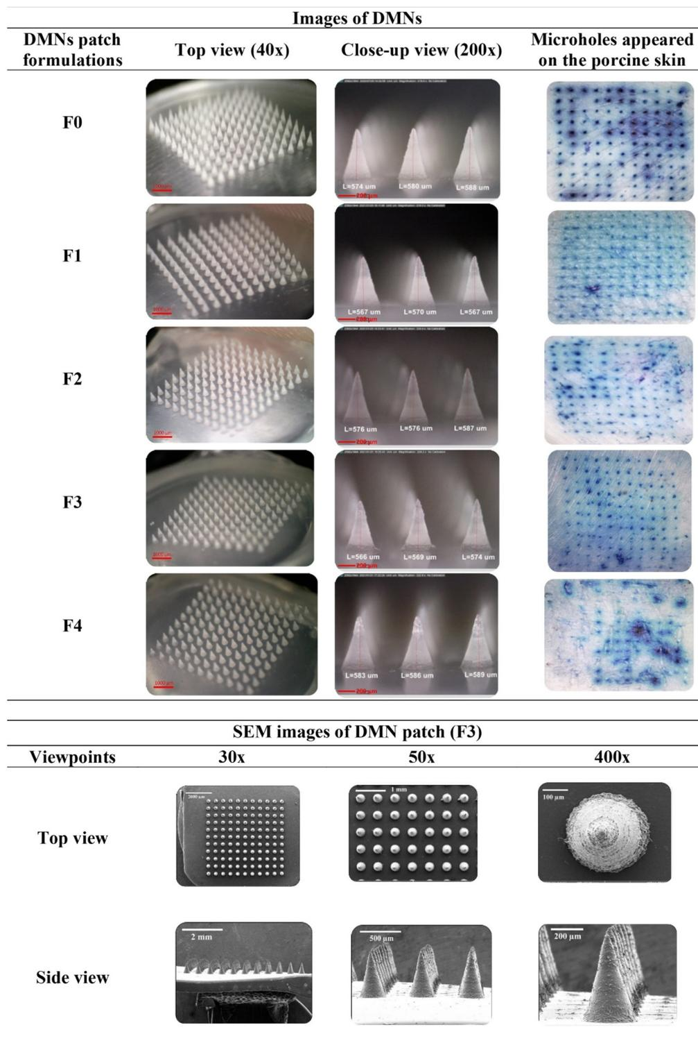
**Fig. 3** Morphology of AA/Res-loaded DMN patches, stained microholes following insertion, and SEM images of 10% AA and 2% Res-loaded DMN patches (F3) from different viewpoints and at different magnifications.
