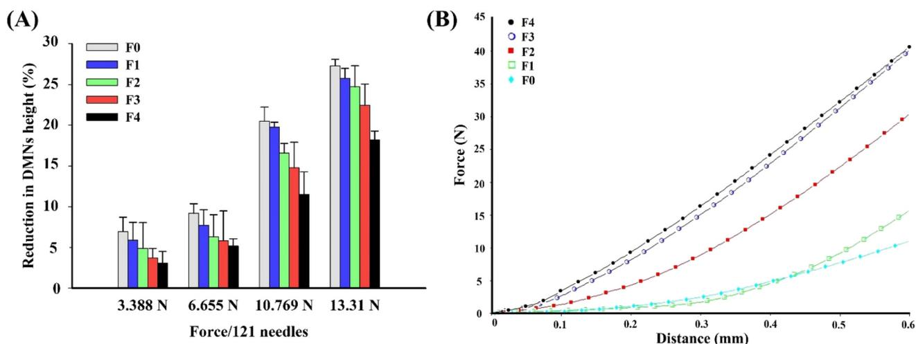
Fig. 4 (A) Percentage height reduction of F0, F1, F2, F3, and F4 DMN formulations following various compression forces applied (mean  $\pm$  SD,  $n = 3$ ). (B) Typical force–displacement curve of the compression force of different DMN formulations.
