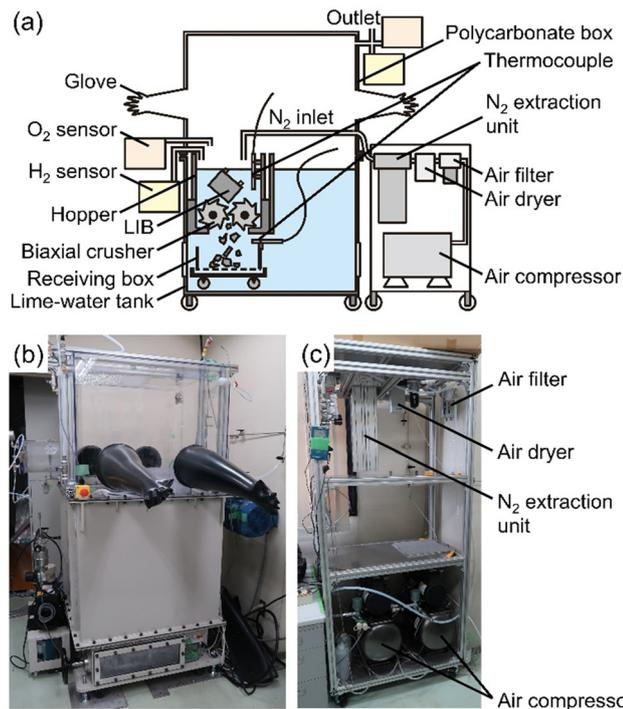
Fig. 2 Equipment for submerged comminution of LIBs in lime water under  $N_2$  flow. (a) Schematic illustration. Photographs of (b) glove box with lime-water tank and (c) setup for  $N_2$  gas supply (maximum flow rate  $22.0 \text{ L min}^{-1}$  @ 99.9%  $N_2$ ,  $56.4 \text{ L min}^{-1}$  @ 99%  $N_2$ ).
