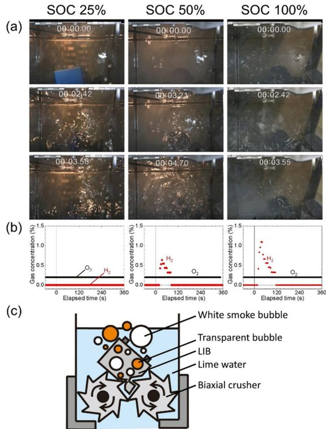
Fig. 3 Observation and analysis of the submerged comminution. (a) Photographs of cell batteries being comminuted. (b) Concentration trend of hydrogen above the water surface and oxygen in the glove box. (c) Schematic illustration of the comminution in lime water for the higher SOC.
