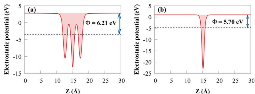
Fig. 5 Work function for (a) the GeI<sub>2</sub> monolayer and (b) C<sub>2</sub>N.
