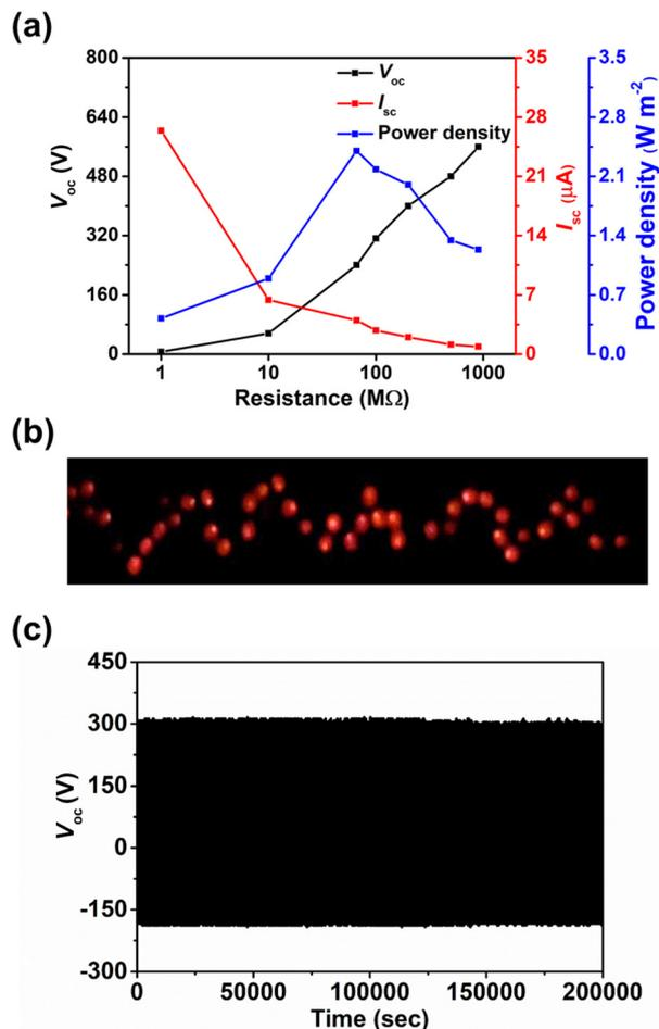
Fig. 7 (a) Output characteristics of resulting TENG as a function of the load resistance. (b) A photograph of 64 LEDs lit up simultaneously by resulting TENG. (c) Evolution of  $V_{oc}$  of resulting TENG as a function of continuous operating cycles under ambient air conditions (25 °C, 50% relative humidity).
