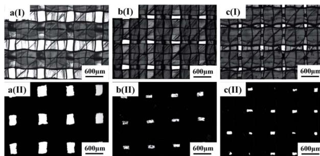
Fig. 2 Microscopic images of the prepared membranes with different pore sizes ((a),  $240 \times 400 \mu\text{m}$ , (b),  $100 \times 240 \mu\text{m}$ , (c),  $100 \times 150 \mu\text{m}$ ; I represents ABS membranes; II represents ABS-Ni membranes).
