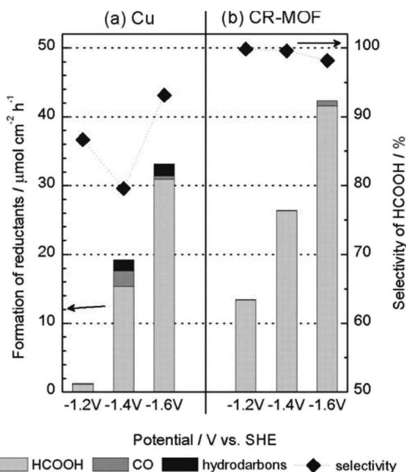
Fig. 8 Contrast between the electrocatalytic performance and selectivity of Hinogami *et al.* (ref. 100). Cu–rubeanic acid MOF and a Cu electrode (ref. 100, ©The Electrochemical Society. Reproduced by permission of IOP Publishing Ltd all rights reserved).
