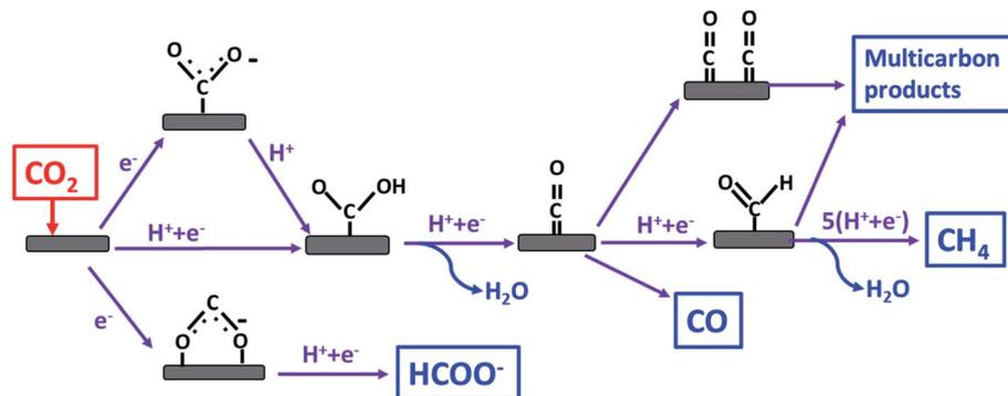
Fig. 1 Scheme of the CO<sub>2</sub> reduction pathway toward different reaction products.
