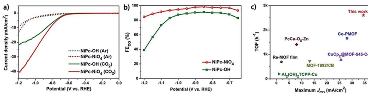
Fig. 7 Electrocatalytic performance of the NiPc-NiO<sub>4</sub> MOF system vs. isolated Ni-Pc (ref. 63). (a) LSV curve comparison in Ar and CO<sub>2</sub> saturated electrolyte. (b) Faradaic efficiencies towards CO formation. (c) Performance comparison vs. other reported CO<sub>2</sub>RR electrocatalytic systems (reproduced with permission from ref. 63, ©2021 Wiley-VCH GmbH).
