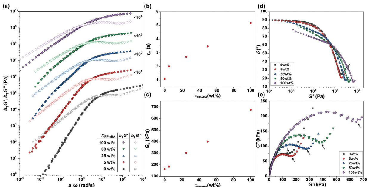
Fig. 3 (a) Master curves of storage ( $G'$ ) and loss ( $G''$ ) moduli for PnBA/PPnBA blended elastomers at the reference temperature of 20 °C. The data are vertically shifted for clarity using the multiplication factors shown in the plot. (b) Relaxation time of the melt ( $\tau_m$ ) and (c) plateau modulus ( $G_N$ ) for the PnBA/PPnBA elastomer blend as a function of PPnBA fraction,  $x_{\text{PPnBA}}$ . (d) van Gurp–Palmen plots and (e) Cole–Cole plots of the PnBA/PPnBA elastomer blends.
