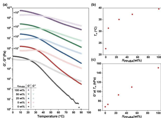
Fig. 2 (a) Temperature-dependence of storage ( $G'$ ) and loss ( $G''$ ) moduli of PnBA/PPnBA blended elastomers with  $\gamma = 1.0\%$  and  $\omega = 10$  rad  $s^{-1}$ . The data are vertically shifted for clarity using the multiplication factors shown in the plot. (b) Melting temperature ( $T_m$ ) and (c)  $G'$  at  $T_m$  of the PnBA/PPnBA elastomer blend as a function of PPnBA fraction ( $x_{PPnBA}$ ).
