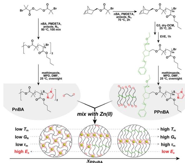
Fig. 1 Conceptual illustration of this study and synthesis of the target polymers. Detailed synthetic procedures are provided in the ESI.†
