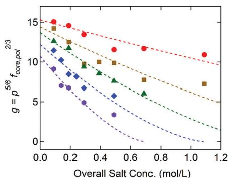
Fig. 5 Dimensionless parameter for the interfacial tension,  $g = \rho^{5/6} f_{\text{core,pol}}^{2/3}$ , as a function of the overall salt concentration for  $G_0 + S$  (purple/hexagons),  $G_{0.32} + S$  (blue/diamonds),  $G_{0.49} + S$  (green/triangles),  $G_{0.76} + S$  (brown/squares), and  $G_{0.95} + S$  (red/circles). The dashed lines are the best fits to the model function of  $g = g_0(1 - c_s/c^*)^{3/2}$ .
