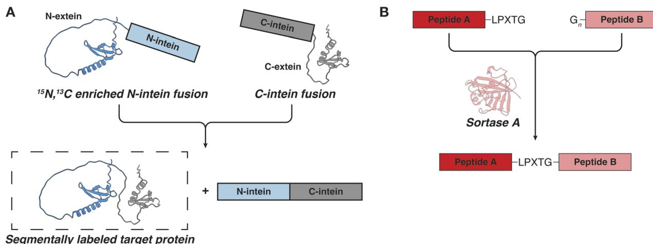
Fig. 3 Approaches for segmental labeling of IDPs for NMR studies. (A) Intein mediated protein *trans*-splicing. (B) Ligation of recombinant or synthetic polypeptides by sortase.
