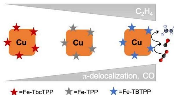
Fig. 8 Schematic representation of the proposed mechanism for **C<sub>2</sub>H<sub>4</sub>** promotion in **Cu<sub>cub</sub>/Fe-Por** tandem catalysts. The C–C coupling enhancement and **C<sub>2</sub>H<sub>4</sub>** promotion correlate with the **Fe-Por** selectivity and conversion rate for **CO**.
