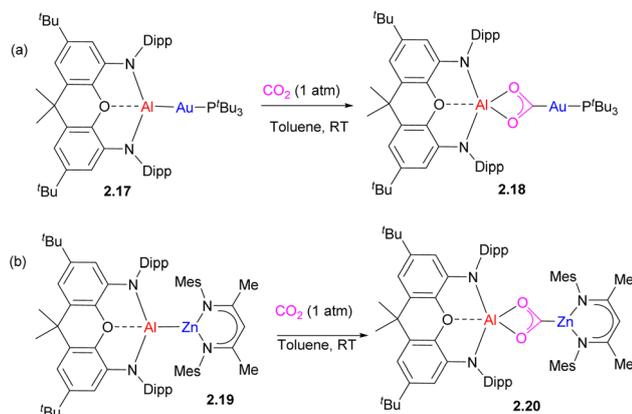
Scheme 9 Bimetallic CO<sub>2</sub> activation of carbon dioxide by (a) Al/Au and (b) Al/Zn complexes.
