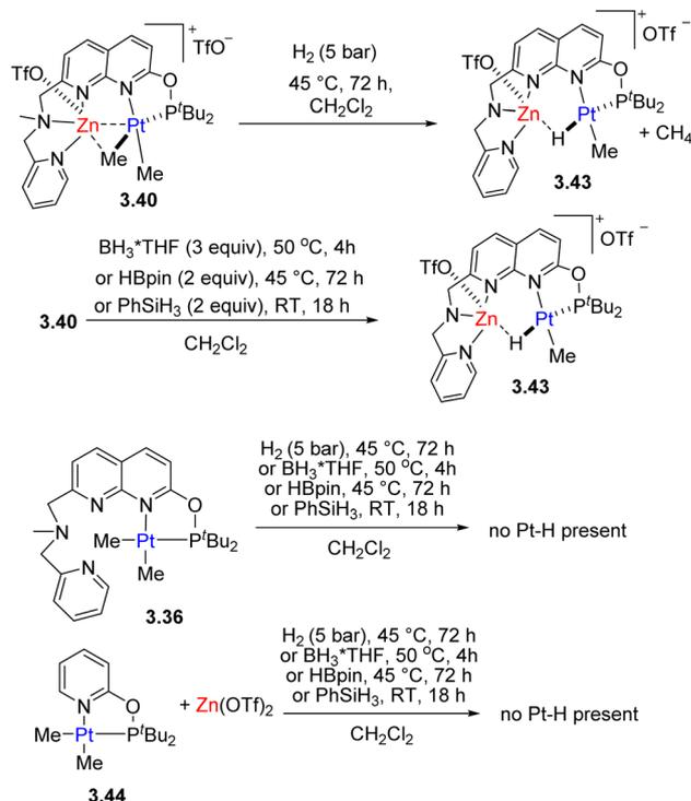
Scheme 33 Reactivity of Pt/Zn complexes and their monometallic analogues in H<sub>2</sub>, Si–H and B–H bond activation.
