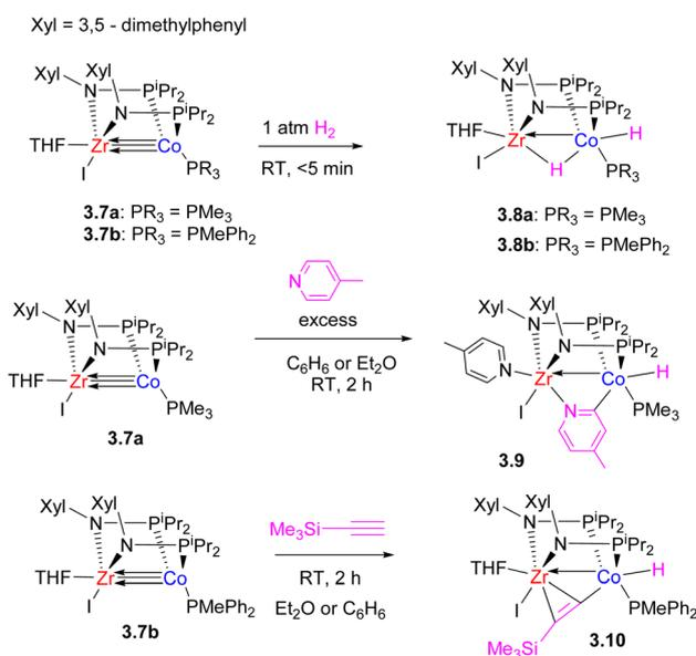
Scheme 16 The reactivity of a bis(phosphinoamido) Zr/Co complex in H<sub>2</sub> and C–H bond activation.
