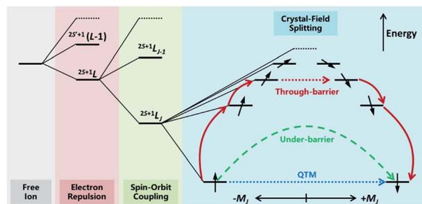
Fig. 2 The energy level splitting of a typical heavy Ln<sup>3+</sup> ion placed in an axial electrostatic crystal field, as well as the possible relaxation pathways. Higher-energy spin states are abbreviated for clarity.
