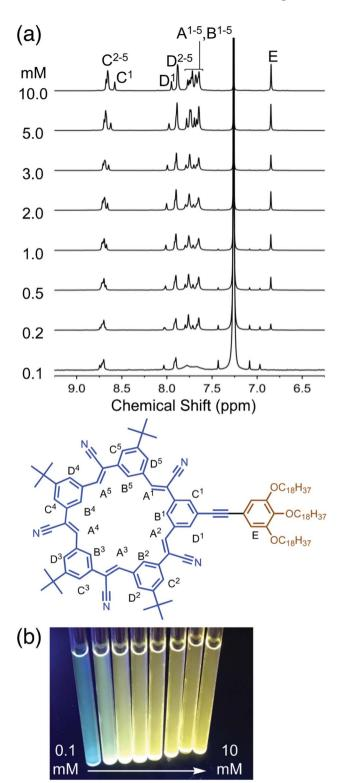
**Fig. 3** Variable concentration studies of **cyanosurf** in organic solution (a) observed using  $^1$ H NMR spectra recorded 0.1–10 mM (CDCl $_3$ , 298 K, 600 MHz) and (b) a photograph of the corresponding NMR tubes recorded under UV light illumination.
