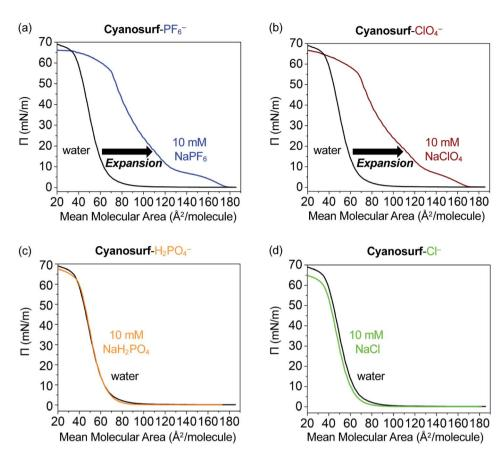
Fig. 4 The  $\Pi$ -A isotherms of the **cyanosurf** molecules on water (black trace) and on a 10 mM aqueous solution of the sodium (Na<sup>+</sup>) salts of (a) hexafluorophosphate (PF<sub>6</sub><sup>-</sup>) (blue trace), (b) perchlorate (ClO<sub>4</sub><sup>-</sup>) (brown trace), (c) dihydrogen phosphate (H<sub>2</sub>PO<sub>4</sub><sup>-</sup>) (orange trace), and (d) chloride (Cl<sup>-</sup>) (green trace), respectively.
