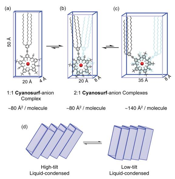
Fig. 6 Molecular models of the supra-amphiphile complexes at the air—water interface as (a) a 1:1 complex, (b) 2:1 complexes with either  $\sim 36^{\circ}$  or (c)  $\sim 108^{\circ}$  rotation angles that are defined by the sterically-geared *tert*-butyl groups on the macrocycles. (d) Tilted arrangements of the supra-amphiphiles.
