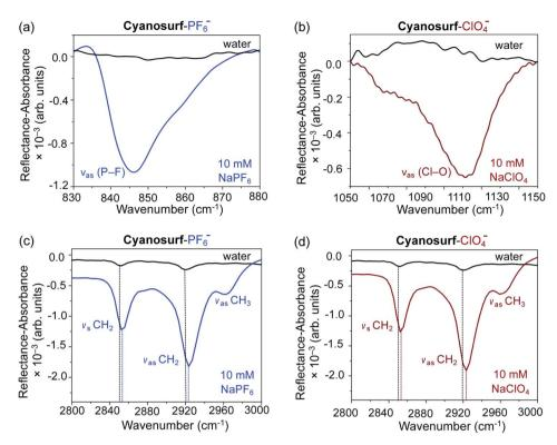
Fig. 7 IRRAS spectra showing cyanosurf reorganization upon anion binding. The spectrum of the cyanosurf molecules on water is shown as a black trace for (a)–(d). The spectra of the cyanosurf molecules with 10 mM of the sodium salts of (a) and (c)  $ClO_4$  (brown) and (b) and (d)  $PF_6$  (blue) at a MMA of 150 Å<sup>2</sup> per molecule.
