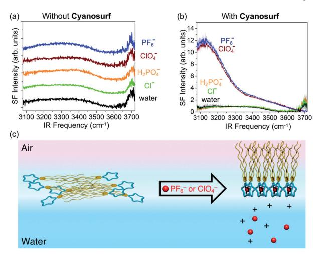
Fig. 8 Sum frequency generation spectra of the: (a)  $H_2O$ ,  $Cl^-$ ,  $H_2PO_4^-$ ,  $PF_6^-$ , and  $ClO_4^-$  aqueous solutions without the **cyanosurf** shown with a baseline offset for clarity, (b) and with the **cyanosurf**. (c) Schematic representation of the anion-induced organization of the **cyanosurf** monolayer. Spectra were obtained after an equilibration time of 10 minutes following the spreading of **cyanosurf** to a constant MMA of 150 Å<sup>2</sup> per molecule.
