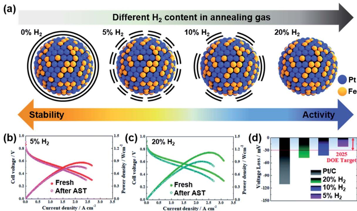
Fig. 5 (a) Difference in the carbon shell depending on annealing conditions; various percentages of H<sub>2</sub> flow were used at 700 °C. *I*-*V* curves before and after accelerated stress tests (ASTs) performed under (b) 5% H<sub>2</sub> and (c) 20% H<sub>2</sub>. (d) Voltage loss at 0.8 A cm<sup>-2</sup> after ASTs. Reproduced from ref. 90 with permission, copyright 2021, the Royal Society of Chemistry.
