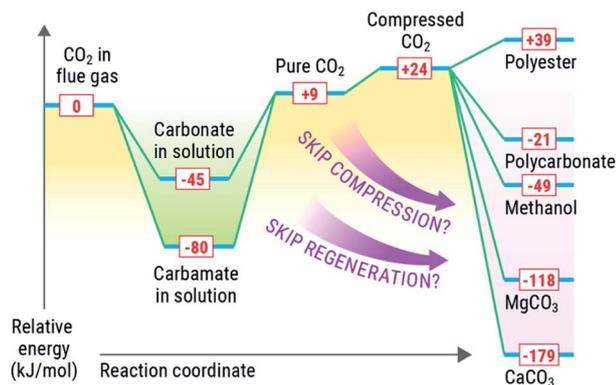
Fig. 3 Conceptual energy comparison for capture and conversion of CO<sub>2</sub>.
