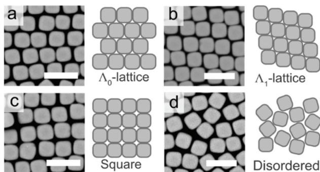
**Fig. 8** The (a)  $\Lambda_0$ -lattice, (b)  $\Lambda_1$ -lattice (c) square lattice, and (d) disordered assembly patterns observed in SEM micrographs. Scale bars represent 2  $\mu\text{m}$ . Reproduced with permission from ref. 95. Copyright 2019 American Chemical Society.
