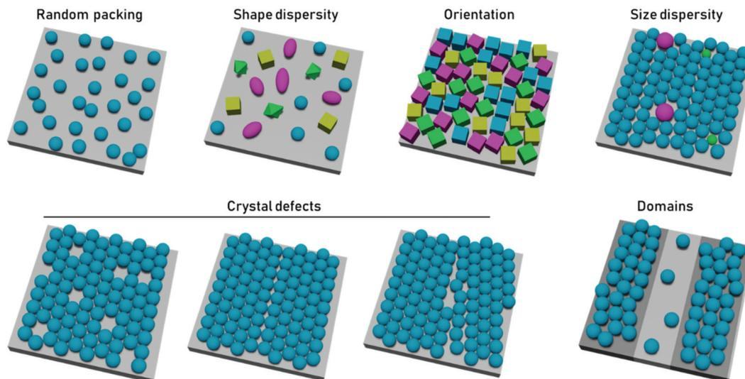
**Fig. 2** The most common sources of disorder are from random, non-close packing, from dispersity in particle shape, orientation, or size, from crystal defects, such as point or line defects and grain boundaries, and from particle placement outside desired domains.
