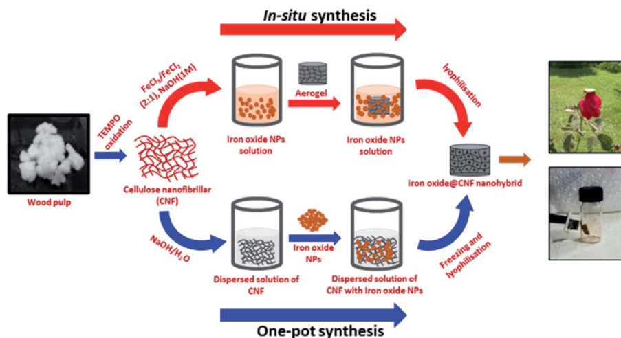
Fig. 1 Schematic representation of the synthesis of the iron oxide@CNF nanohybrid by in situ and one-pot synthesis.
