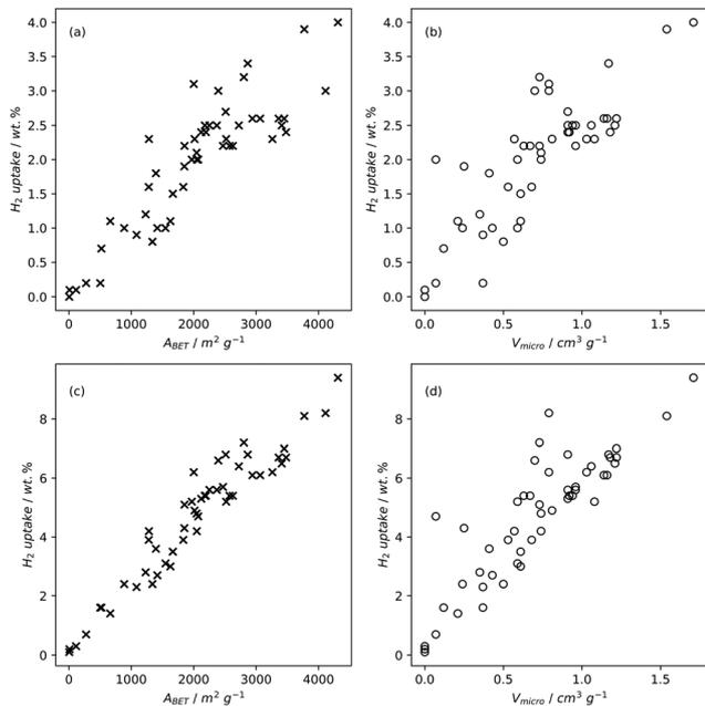
Fig. 2 H<sub>2</sub> uptake of carbons at  $-196\text{ }^{\circ}\text{C}$  and 1 bar (a) and (b) or 20 bar (c) and (d) as a function of BET surface area (a) and (c) or micropore volume (b) and (d).<sup>79,82,83,196,220,221</sup>
