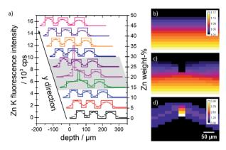
Fig. 5 (a) Quantified ZnO concentration values (lines) with corresponding measurement data (scatter) at  $x=0~\mu m$ . The depth profiles are displaced in x- and y-direction for better clarity. The area of the dent is marked with a grey shaded area. (b and c) Absorption values  $x=0~\mu m$  for an idealized homogeneous sample (b) and a sample with a dent (c). (d) Difference values in percent.
