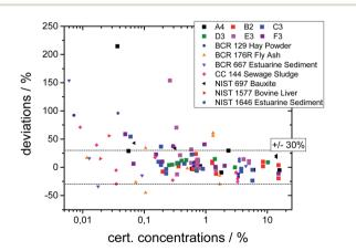
Fig. 3 Deviations of the quantified concentration values to the certified values as a function of certified values.
