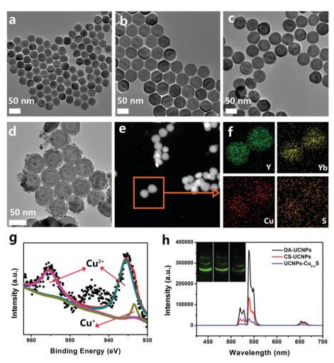
Fig. 1 TEM images of (a) NaYF<sub>4</sub>:Yb/Er, (b) NaYF<sub>4</sub>:Yb/Er@NaYF<sub>4</sub>:Yb (UCNPs), (c) CS-UCNPs, and (d) UCNPs-Cu<sub>2-x</sub>S. (e) HAADF-STEM image of UCNPs-Cu<sub>2-x</sub>S and (f) the corresponding element mappings. (g) XPS of Cu in UCNPs-Cu<sub>2-x</sub>S. (h) UCL spectra of OA-UCNPs, CS-UCNPs, and UCNP-Cu<sub>2-x</sub>S excited by a 980 nm NIR laser. Insets are the corresponding digital photographs of the solutions irradiated by the 980 nm NIR laser.
