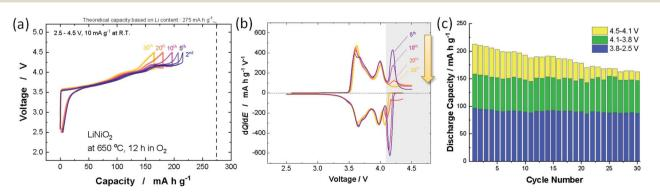
Fig. 1 (a) Galvanostatic charge/discharge curves of LiNiO<sub>2</sub> at a rate of 10 mA  $g^{-1}$ , (b) differential dQ/dE plots obtained from (a), and (c) variations in discharge capacities with different voltage ranges.
