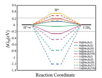
Fig. 7 Calculated Gibbs free energy diagram for the HER at different sites for Ni@Mo<sub>2</sub>B<sub>2</sub> and Cu@Mo<sub>2</sub>B<sub>2</sub> for a hydrogen coverage of 1/16. The two horizontal black dashed lines correspond to  $|\Delta G_H| = 0.2$  eV.
