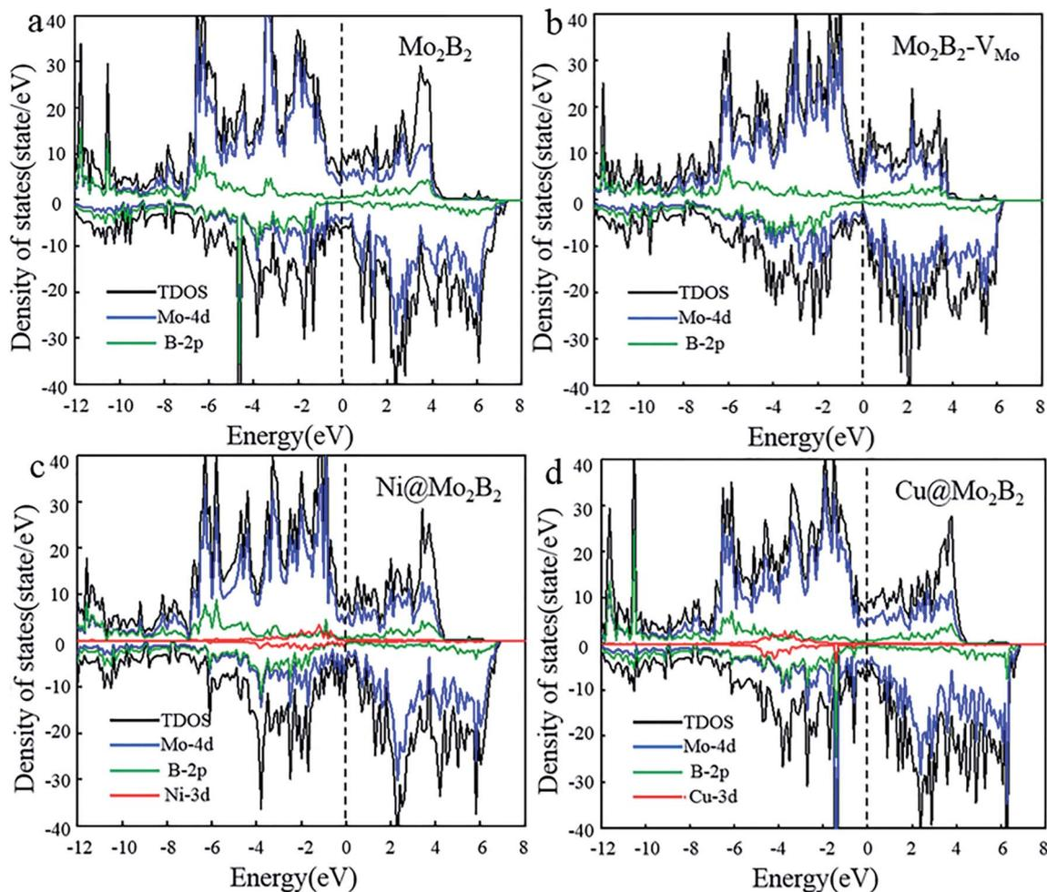
Fig. 2 The total density of states (TDOS) and the projected density of states (PDOS) of (a) pristine  $\text{Mo}_2\text{B}_2$ , (b)  $\text{Mo}_2\text{B}_2\text{-V}_{\text{Mo}}$ , (c)  $\text{Ni@Mo}_2\text{B}_2$  and (d)  $\text{Cu@Mo}_2\text{B}_2$ , where the Fermi level is set to 0 eV.
