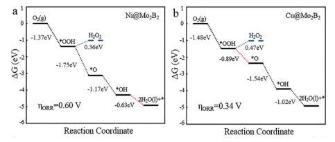
Fig. 5 The Gibbs free energy diagrams for the 4e<sup>-</sup> and 2e<sup>-</sup> ORR processes of (a) Ni@Mo<sub>2</sub>B<sub>2</sub> and (b) Cu@Mo<sub>2</sub>B<sub>2</sub> at site I, where the blue lines represent the 2e<sup>-</sup> ORR process, the black lines represent the 4e<sup>-</sup> ORR process, and the red dashed lines represent the most energy-consuming step of the ORR.
