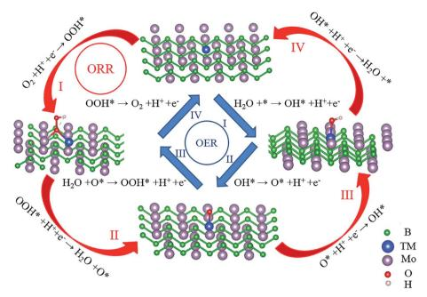
Fig. 3 Elementary reaction steps of the OER and ORR process for TM@Mo<sub>2</sub>B<sub>2</sub> at site I.
