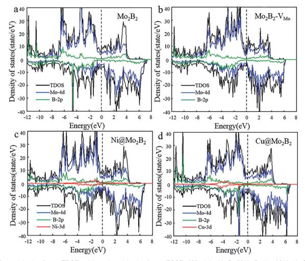
Fig. 2 The total density of states (TDOS) and the projected density of states (PDOS) of (a) pristine Mo<sub>2</sub>B<sub>2</sub>, (b) Mo<sub>2</sub>B<sub>2</sub>-V<sub>Mo</sub>, (c) Ni@Mo<sub>2</sub>B<sub>2</sub> and (d) Cu@Mo<sub>2</sub>B<sub>2</sub>, where the Fermi level is set to 0 eV.
