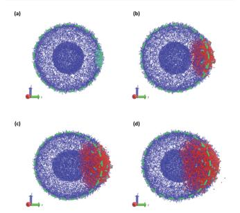
Fig. 10 Vesicle morphology at (a) t = 0, (b) t = 75, (c) t = 150, and (d) t = 250 while a chemical reaction produces  $S_B$  that swells the vesicle. Blue particles represent the monomers in the A-block of the polymer, cyan particles represent the enzyme (E) beads, and red particles represent SB solvent particles. Monomers in the B-block and other solvent particles are not shown for clarity. The dashed green circle indicates the initial vesicle circumference as a guide to the eye.
