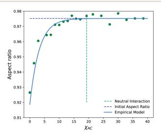
Fig. 14 Aspect ratio (AR) as a function of the interaction parameter, χ<sub>AC</sub>, of newly created monomers on the solvophobic block. The neutral interaction point occurs when C particles can no longer distinguish between A and B beads, i.e. when  $\chi_{AC} = \chi_{BC}$ .
