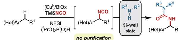
Fig. 1 Copper-catalyzed benzylic C(sp 3 )–H isocyanation/amine coupling. (A) Drug candidates embedding benzylic urea. (B) Two possible one-pot synthetic approaches toward ureas from benzylic C–H substrates. (C) Strategy for high-throughput synthesis of ureas. NFSI, N -fluorobenzenesulfonimide; BiOx, 2,2'-bis(oxazoline); TMSNCO, (trimethylsilyl)isocyanate.
