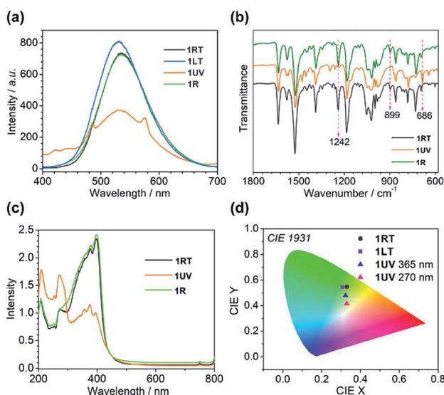
Fig. 4 (a) The emission spectra excited at 365 nm for **1RT**, **1LT**, **1UV** and **1R**. (b) The IR spectra of **1RT**, **1UV** and **1R**. (c) The absorption spectra of **1RT**, **1LT**, **1UV** and **1R** in the solid state. (d) The 1931 CIE graphs of **1RT**, **1LT** and **1UV**.
