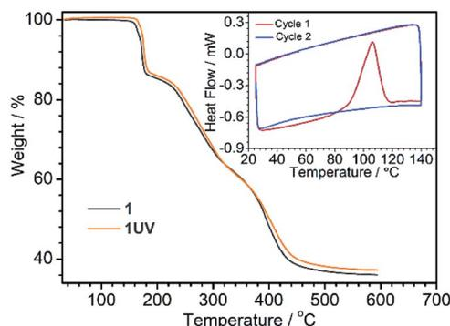
Fig. 5 TGA curves of **1** (grey) and **1UV** (yellow) measured under a nitrogen flow at a heating rate of 5 °C min<sup>-1</sup>. Inset: the DSC curves for **1UV** between 25 and 140 °C at a scan speed of 5 °C min<sup>-1</sup> for two cycles.
