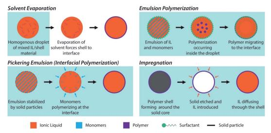
Fig. 2 Schematic representations of the different methods used for the preparation of encapsulated ILs.
