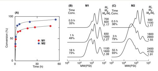
Fig. 1 ADMET polymerization of sequence-regulated telechelic diene oligomers (M1 and M2) ([M]<sub>0</sub>/[G2]<sub>0</sub> = 400) in bulk at 50 °C. Time-conversion curves (A) and SEC curves of the products obtained from M1 (B) and M2 (C).
