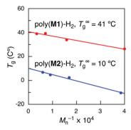
Fig. 6  $T_{\rm g}$  values of hydrogenated poly(M1) (poly(M1)-H<sub>2</sub>) and poly(M2) (poly(M2)-H<sub>2</sub>) with various molecular weights and  $T_{\rm g}^{\infty}$  values estimated using the Flory-Fox equation.
