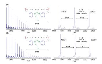
Fig. 4 MALDI-TOF-MS spectra of poly(M2) (A) and the hydrogenated poly(M2) (poly(M2)-H<sub>2</sub>) (B).
