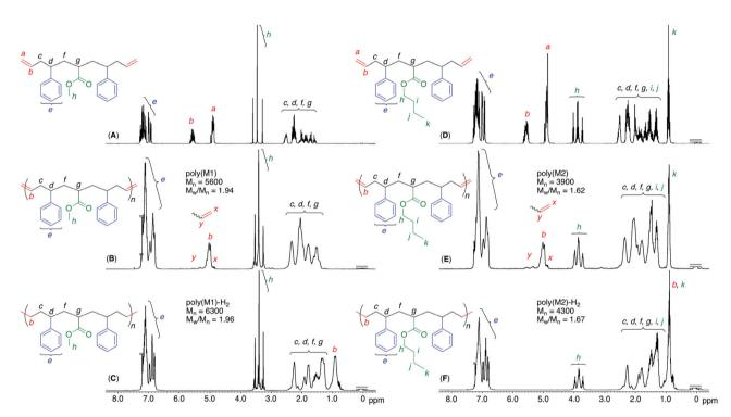
Fig. 3 <sup>1</sup>H NMR spectra (CDCl<sub>3</sub>, 25 or 55 °C) of sequence-regulated telechelic diene oligomers (M1 and M2) (A and D), sequence-regulated polymers obtained *via* ADMET polymerization of M1 and M2 (B and E), and the hydrogenated polymers (C and F).
