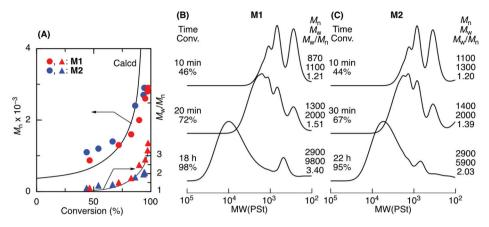
Fig. 2 ADMET polymerization of sequence-regulated telechelic diene oligomers (M1 and M2) ([M]<sub>0</sub>/[G2]<sub>0</sub> = 1500/3.75 mM) in tetralin at 50 °C.  $M_n$  and  $M_w/M_n$  vs. monomer conversion plots (A) and SEC curves the products obtained from M1 (B) and M2 (C).
