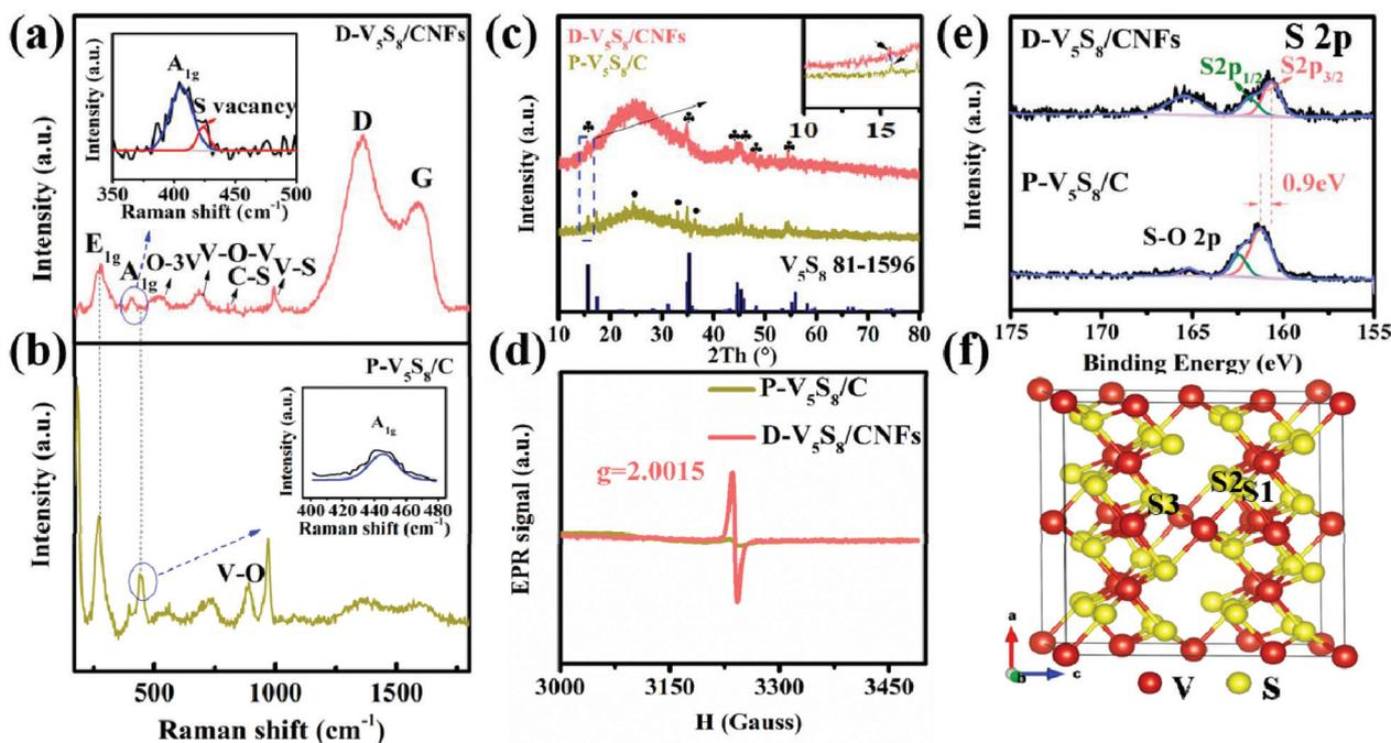
**Fig. 2** (a and b) Raman spectra, (c) XRD pattern, (d) EPR spectrum, and (e) XPS analysis of the P-V<sub>5</sub>S<sub>8</sub>/C and D-V<sub>5</sub>S<sub>8</sub>/CNF samples. (f) Schematic illustration of the atom arrangements in V<sub>5</sub>S<sub>8</sub>; note that S1, S2, and S3 represent the possible sulfur defects.
