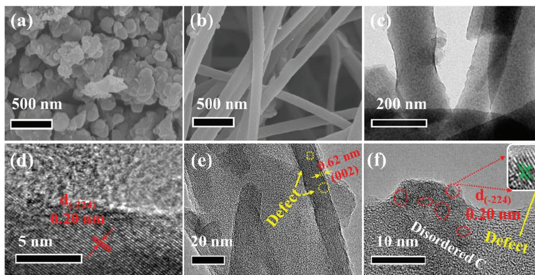
**Fig. 1** SEM morphology of (a)  $\text{P-V}_5\text{S}_8/\text{C}$  and (b)  $\text{D-V}_5\text{S}_8/\text{CNFs}$ . (c) TEM image of  $\text{D-V}_5\text{S}_8/\text{CNFs}$ . The corresponding HRTEM images of (d)  $\text{P-V}_5\text{S}_8/\text{C}$  and (e and f)  $\text{D-V}_5\text{S}_8/\text{CNFs}$ . Note that the inset of (f) shows the relevant enlargement of the dashed box (red).
