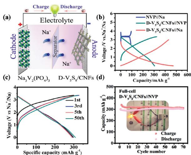
Fig. 5 The energy storage performance of a D- $V_5S_8$ /CNF full cell. (a) Working mechanism of the full cell. (b) Typical charge–discharge curves of the NVP cathode, the D- $V_5S_8$ /CNF anode and the D- $V_5S_8$ /CNFs//NVP full cell. (c) Galvanostatic charge/discharge profiles. (d) Cycling performance of the D- $V_5S_8$ /CNFs//NVP full cell at a current density of 500 mA g<sup>-1</sup>. Inset of (d): an LED lightened by the flexible D- $V_5S_8$ /CNFs//NVP full battery.
