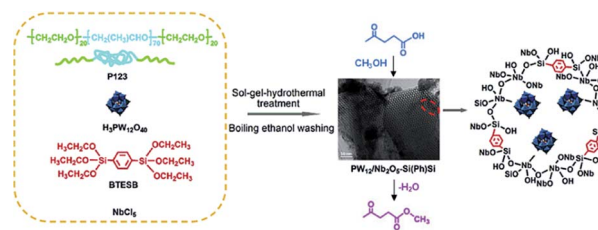
Fig. 8 Preparation route for phenylene-bridged 2D ordered mesoporous PW 12 /Nb 2 O 5 -Si(Ph)Si and the catalytic reaction. 84 Reproduced with permission. 84 Copyright 2016, Elsevier.
