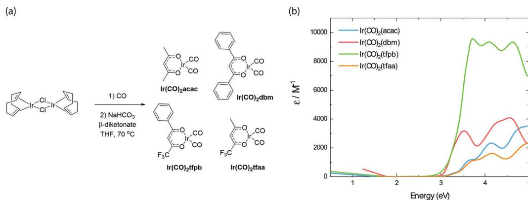
Fig. 1 (a) Synthesis scheme of  $\text{Ir}(\text{CO})_2(\beta\text{-diketonate})$  complexes. (b) Absorbance spectra of the complexes in solution, scaled by their respective molar absorption coefficients.
