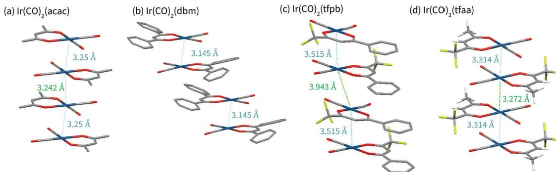
Fig. 3 Schematic of the crystal structures of (a)  $\text{Ir}(\text{CO})_2\text{acac}$ , (b)  $\text{Ir}(\text{CO})_2\text{dbm}$ , (c)  $\text{Ir}(\text{CO})_2\text{tfpb}$ , (d)  $\text{Ir}(\text{CO})_2\text{tfaa}$ , obtained via single-crystal X-ray diffraction. Note that (b) and (c) have two molecules in each asymmetric unit. For all complexes, four molecules are shown to illustrate packing along the axis perpendicular to the plane of the molecules.
