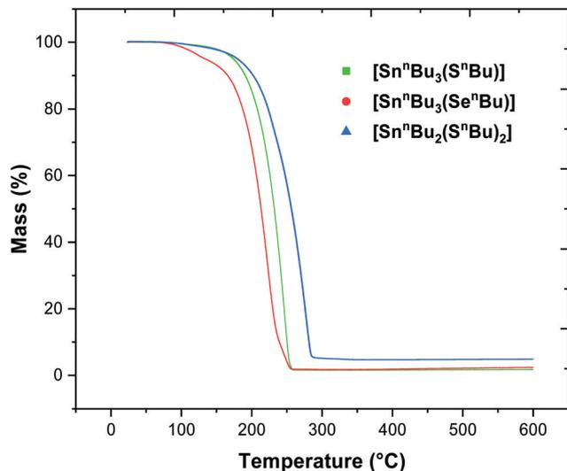
Fig. 1 TGA profiles for (1) (green), (2) (blue) and (3) (red). The TGA experiments were conducted with a temperature ramp rate of  $5\text{ }^{\circ}\text{C min}^{-1}$  and a constant flow of argon gas at a flow rate of  $30\text{ mL min}^{-1}$ .
