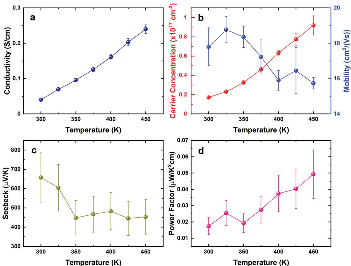
Fig. 9 Electrical properties SnS thin films. Resistivity (a), Hall mobility and carrier concentration (b), Seebeck coefficient (c), and power factor (d) of the films shown with temperature from 300–450 K.
