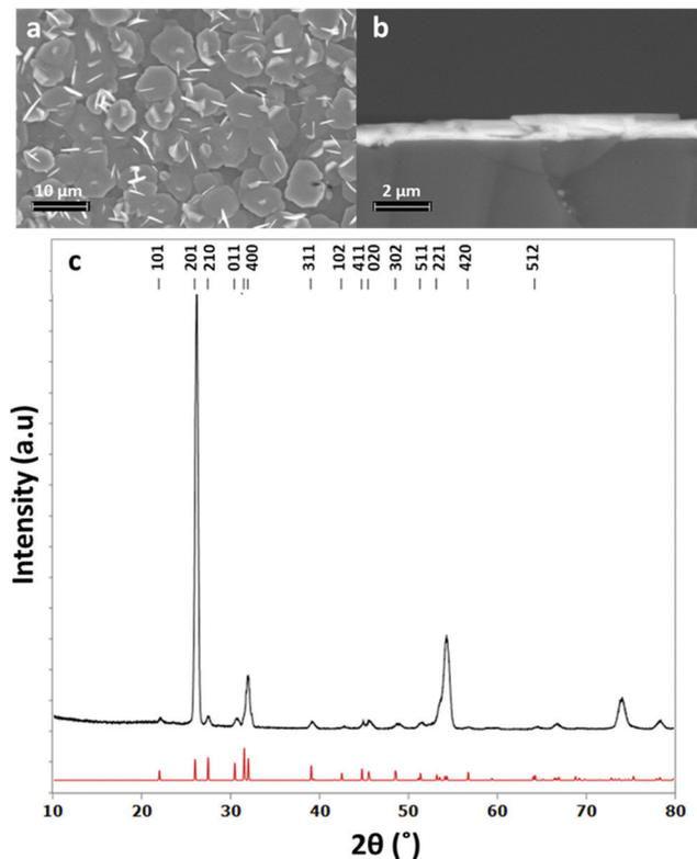
Fig. 4 Top down SEM image (a), cross sectional SEM image (b) and grazing incidence XRD pattern (c) for SnS thin film obtained by low pressure CVD using  $[\text{Sn}^{\text{IV}}\text{Bu}(\text{S}^{\text{IV}}\text{Bu})_2]$  (red = XRD pattern for bulk  $\text{SnS}^{48}$ ) with a thickness of around 700 nm.
