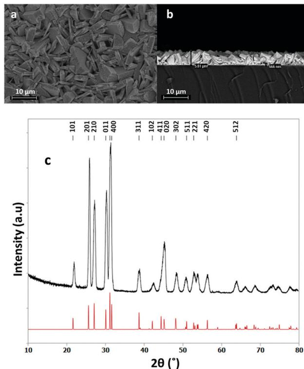
Fig. 2 Top down SEM image (a), cross sectional SEM image (b) and grazing incidence XRD pattern (c) for SnS thin film obtained by low pressure CVD using (2) (red = XRD pattern for bulk SnS<sup>48</sup>) with a thickness of *ca.*  $6\text{ }\mu\text{m}$ .
