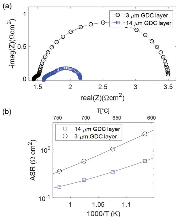
Fig. 7 (a) Impedance spectra of symmetrical cells with 3 and 14  $\mu\text{m}$  GDC layer thickness tested at 600  $^{\circ}\text{C}$  in 7% CO in  $\text{CO}_2$  atmosphere. (b) Arrhenius plot of the ASR.
