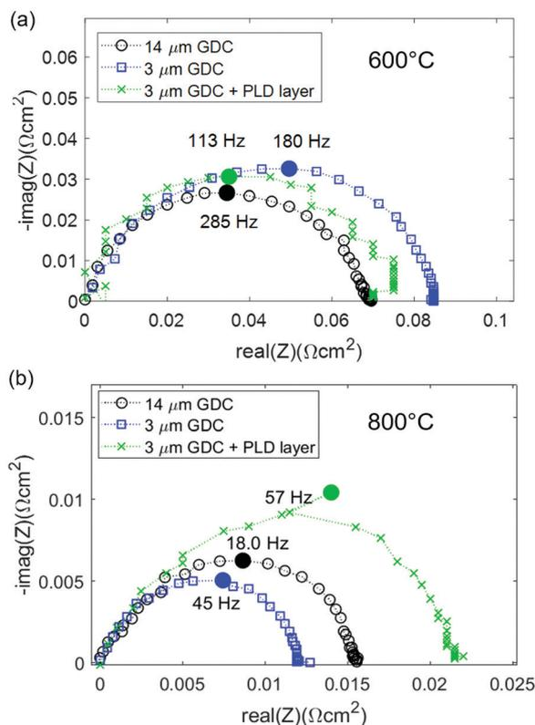
Fig. 4 (a) Impedance spectra of different GDC anodes at (a) 600  $^{\circ}\text{C}$  and (b) 800  $^{\circ}\text{C}$ . The high frequency offset was subtracted from all spectra for the sake of easier comparability.
