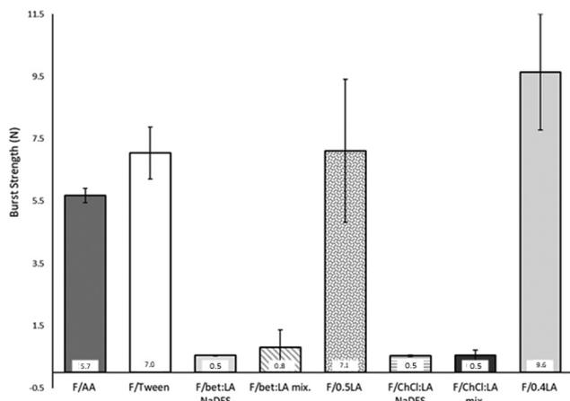
Fig. 1 Burst strength results of the different films.
