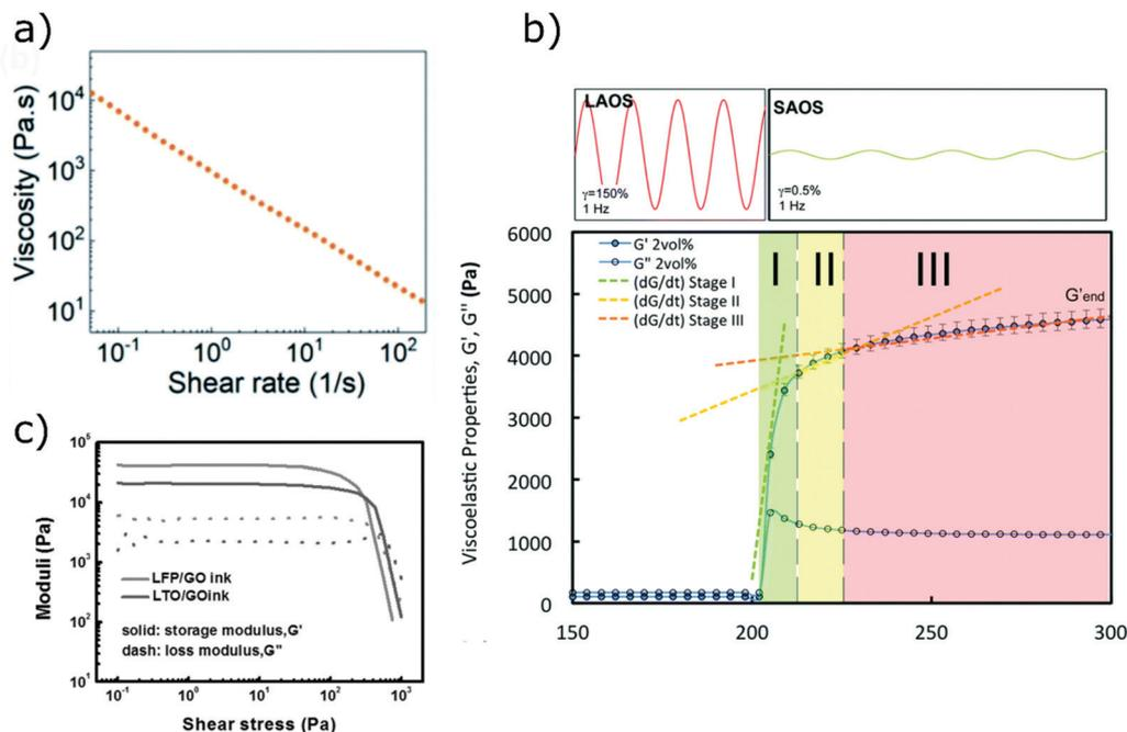
Fig. 7 Experimental data showing the ideal rheological behaviour of inks for DIW: (a) shear thinning flow behaviour (adapted with permission from ref. 149, Published by The Royal Society of Chemistry); (b) quick recovery of the storage modulus after large amplitude oscillatory shear (adapted with permission from ref. 36, published by The Royal Society of Chemistry 2019); (c) solid-like response below the yield stress (adapted with permission from ref. 92, Copyright 2016 John Wiley and Sons).
