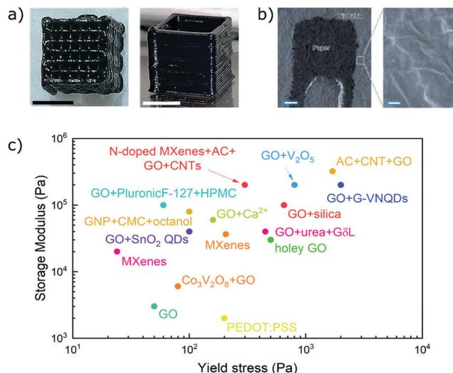
**Fig. 10** (a and b) Pictures of structures printed from  $\text{Ti}_3\text{C}_2\text{T}_x$  inks (adapted with permission from ref. 73, Copyright 2019 John Wiley and Sons, and from ref. 24, Copyright 2019 Springer Nature); (c) plot comparing the storage modulus and yield stress of DIW inks based on graphene oxide and MXenes (references in Table 1).
