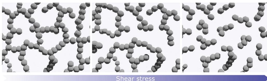
Fig. 5 Microstructure evolution inside a colloidal gel made of a percolated particle network at increasing level of stress.
