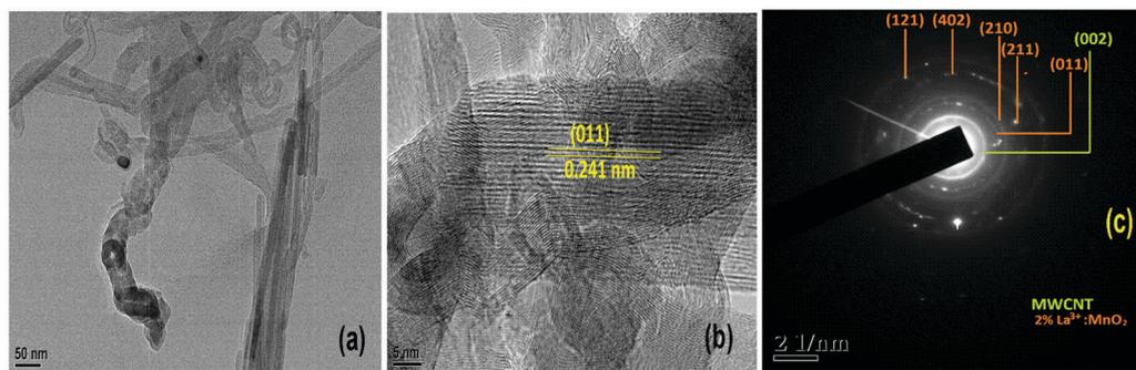
Fig. 6 (a) TEM image; (b) HRTEM image showing a single 2 mol% La<sup>3+</sup>:MnO<sub>2</sub> attached to CNT; and (c) SAED pattern of 2La-MnO<sub>2</sub>-CNT.
