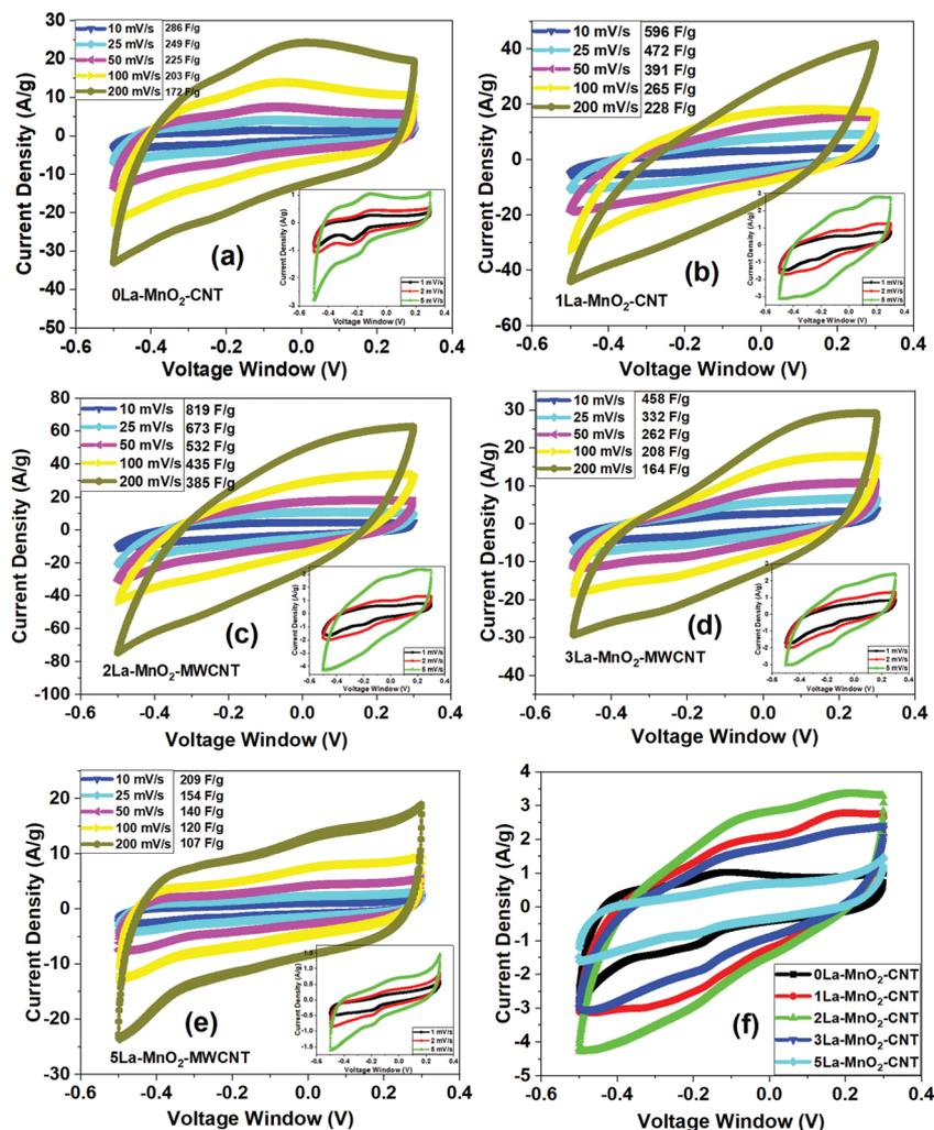
Fig. 7 CV curves of 0La-MnO<sub>2</sub>-CNT (a) and various La-doped MnO<sub>2</sub>-CNT hybrids (b–e) at varying scan rates; (insets of (a–e) show the curves at low scan rates); (f) comparative CV curves of all the samples at 5 mV s<sup>-1</sup> scan rate.
