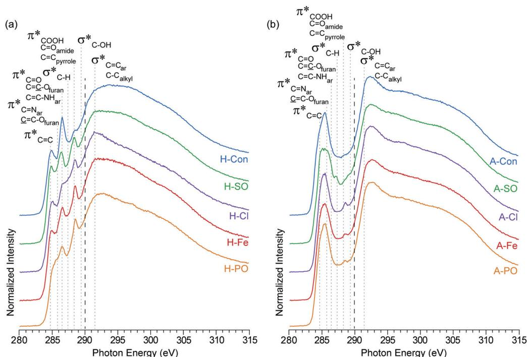
Fig. 3 NEXAFS carbon K-edge spectra of (a) hydrothermal carbons (H-) and (b) activated hydrothermal carbons (A-). Functional group locations for the main C1s  $\rightarrow \pi^*$  and C1s  $\rightarrow \sigma^*$  are added for reference and based on previous NEXAFS work on hydrothermal carbons.<sup>17</sup> The long dashed lines represent the position of the arctangent step function at 290.0 eV.
