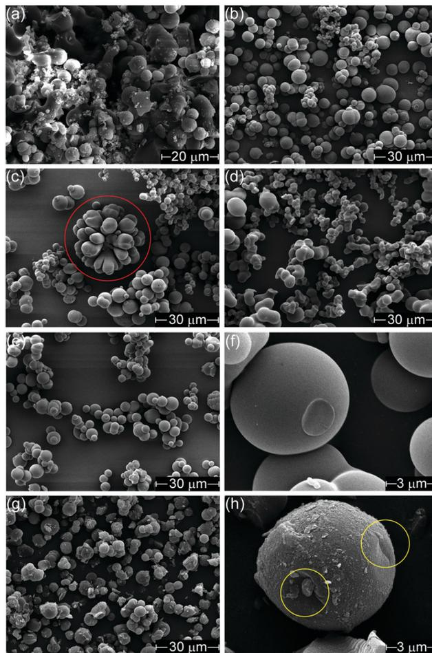
Fig. 1 SEM images of (a) H-Con at 4000 $\times$  (b) H-Cl (c) H-Fe with flower shape outlined in red, (d) H-PO, (e) H-SO, (f) H-SO at 24 000 $\times$ , (g) A-SO and, (h) A-SO at 24 000 $\times$  with removed sections outlined in yellow. Images were taken at 3000 $\times$  magnification, unless otherwise specified.
