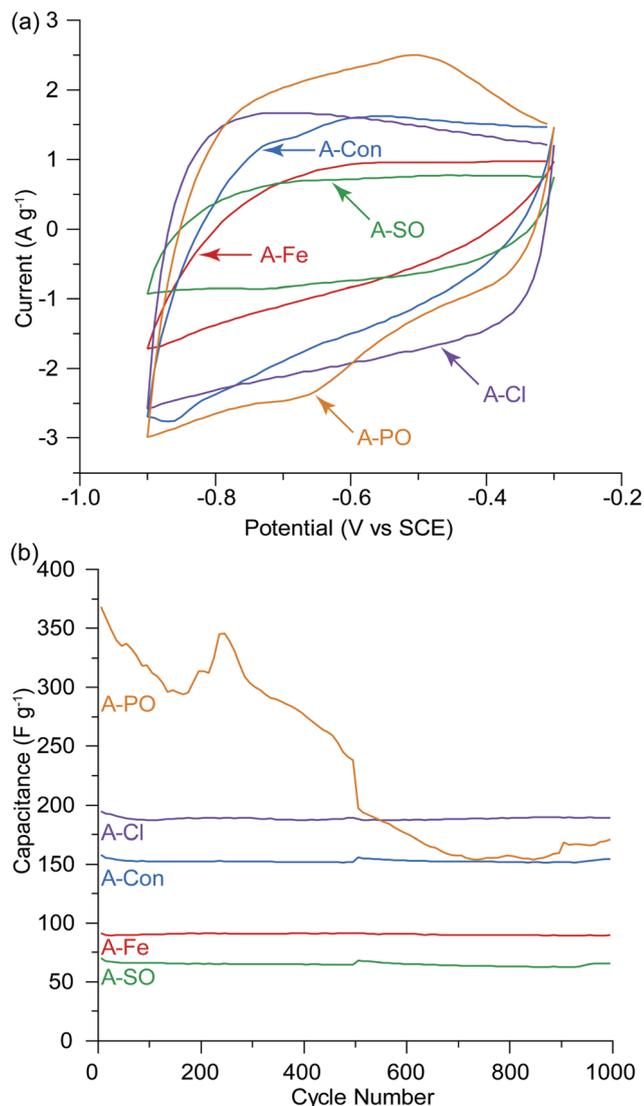
Fig. 5 (a) Cyclic voltammograms at the 500th cycle before the SPECS experiment, (b) capacitance per cycle over 1000 cycles, 10 mV s<sup>-1</sup> in 1 M KOH. The SPECS experiment was conducted at the 500th cycle, hence the slight discontinuity in the capacitance at cycle 500. Decomposition of the electrode/electrolyte was observed for A-PO.
