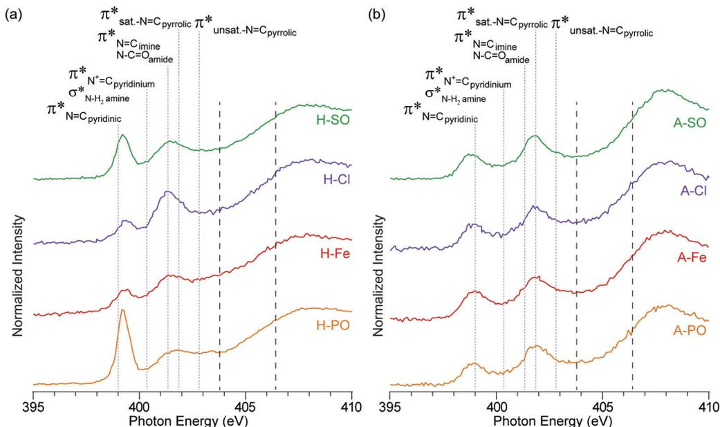
Fig. 4 NEXAFS nitrogen K-edge spectra of (a) hydrothermal carbons and (b) activated hydrothermal carbons. Functional group locations for the main  $N1s \rightarrow \pi^*$  and  $N1s \rightarrow \sigma^*$  are added for reference and based on previous NEXAFS work on hydrothermal carbons.<sup>17</sup> The long dashed lines represent the position of the arctangent step function at 403.9 eV and 406.5 eV.
