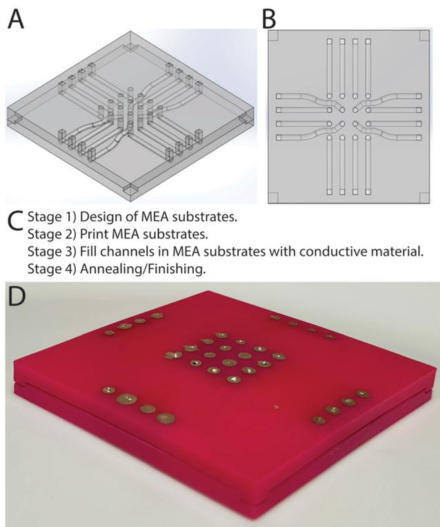
**Fig. 1** (A) CAD model of MEA including cutouts on the bottom half and extrusions on the top half in the corresponding positions to clip the halves together, ensure alignment of the electrodes and ensure the MEA could be handled easily in the laboratory. (B) Top view of CAD model of MEA. (C) Summary of the MEA production process. (D) Photograph of a silver contact MEA (sides 50 mm, height 3 mm).
