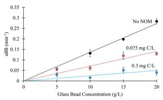
Fig. 3 Influence of GB concentration, B, and SRNOM concentration on the pseudo first order rate constant,  $\alpha\beta B$ . Error bars represent standard deviation of replicates. Linear trendlines fit through the origin are shown as eye-guides.
