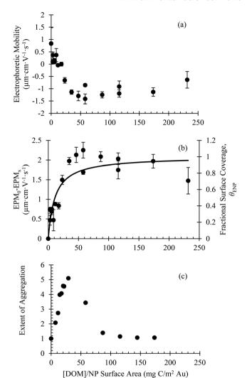
Fig. 2 (a) Electrophoretic mobility of bPEI-AuNPs (5 mg L<sup>-1</sup>); (b) change in electrophoretic mobility and fractional surface coverage  $(\theta_{\rm ENP})$  of bPEI-AuNPs (5 mg L<sup>-1</sup>); and (c) extent of homoaggregation of bPEI-AuNPs (2 mg L<sup>-1</sup>) in the presence of SRNOM. Error bars represent one standard deviation of replicates. Solution conditions included 1 mM HEPES, 20 mM NaCl and varying SRNOM concentrations.
