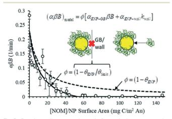
Fig. 5 Experimentally measured pseudo first-order heteroaggregation rate constants  $(\alpha\beta B)$  for collisions between bPEI AuNPs and glass beads and comparison with model predictions.
