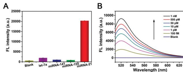
Fig. 3 (A) Selectivity of the proposed strategy for miR-21 and other interfering substances. The error bars represent the standard deviation of three independent measurements. (B) FL responses of different concentrations of miR-21 in 10% actual human serum.
